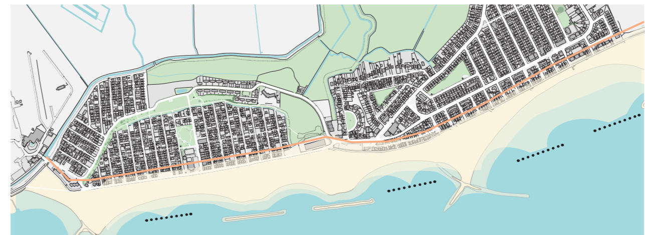
Fig. C42. Map indicatively showing Option C, with reshaped beach and potential locations of new rock groynes (dotted)
