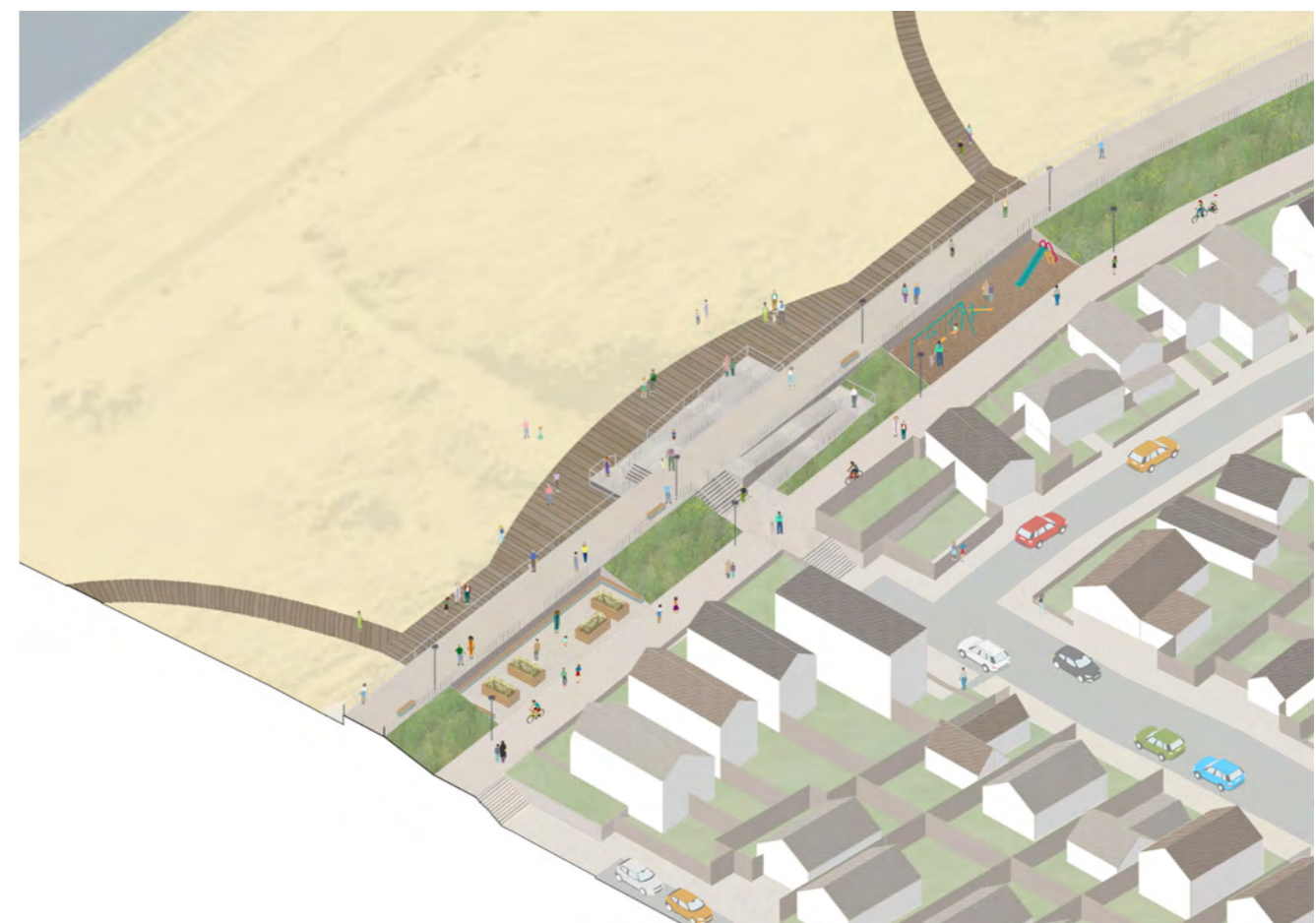
Fig. 70. Isometric sketch showing the main elements of the seafront design strategy along the Village seafront
